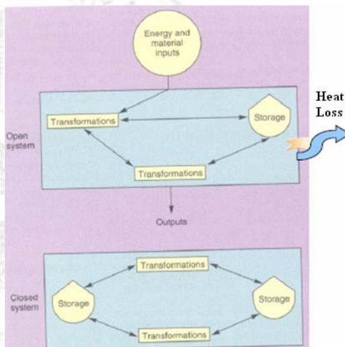
**Fig. 1: Flows in Open and Closed System**
